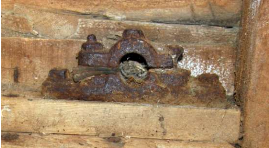
Bearing housing for a horse driven grinding machine still operating post 1942.
